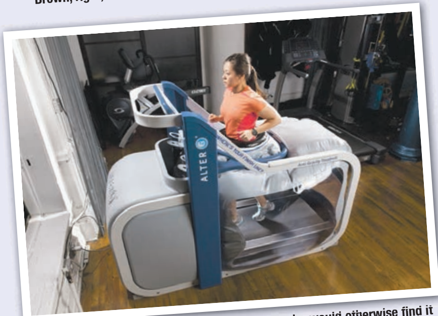
The AlterG Anti-Gravity Treadmill helps people who would otherwise find it difficult to run. The inflatable balloon allows them to run at a lower perceived weight. Physical therapy clinics in Berlin, Bennington and Burlington have the AlterG.
